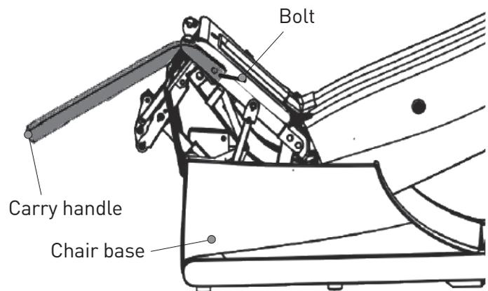
*Attach carry handle as shown; slide bolt through carry handle and into frame.*
